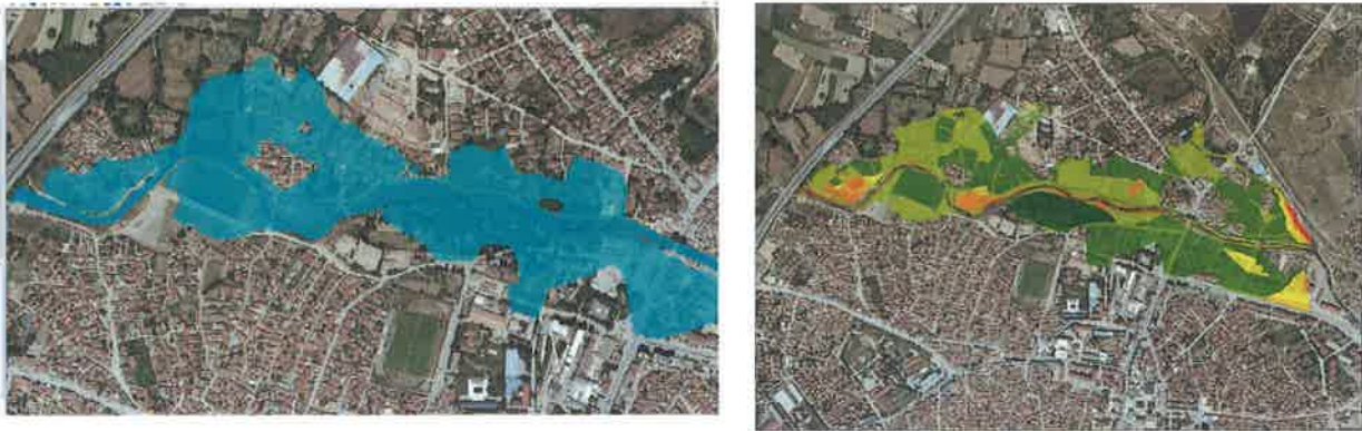
Figure 2. Outputs of the flood risk model: a) Simulation of flooded area by an event with a return period of 100 years; b) Flood risk map with different damage levels based on land-use structure (right)
